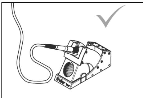
**Always place the soldering tool in the safety rest while not in use.**
